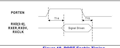
Figure 18. PORT Enable Timing
